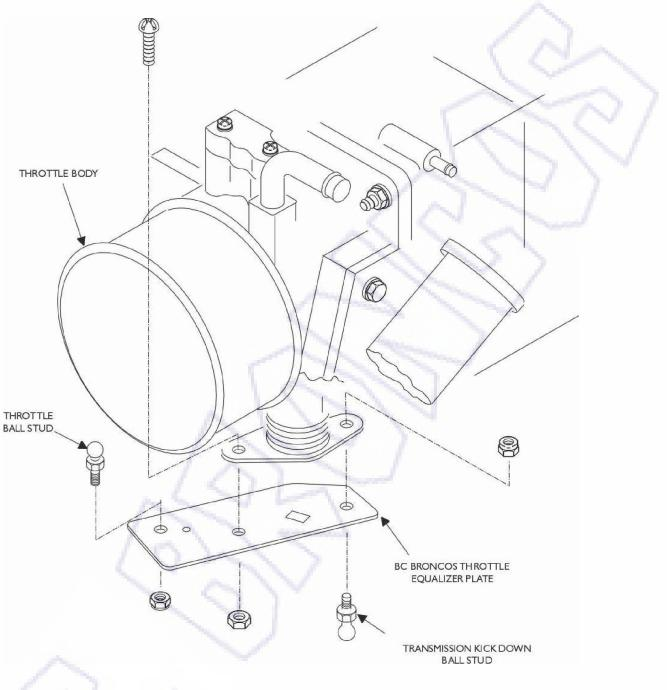
Step 3. Mount the BC Broncos Throttle equalizer and ball studs as shown.
